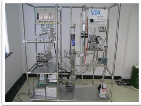
Thin film evaporation (with rectification system) evaporative power: 3kg/h Rectification capacity: 0.5kg~1kg/h
