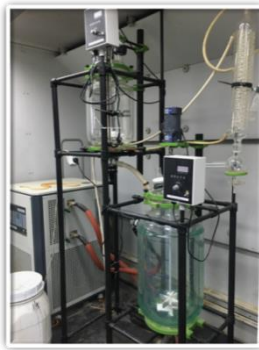
50L reaction equipment Used for pilot synthesis
